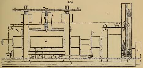
In these rolls a new description of tightening-down gear has been designed, in order to obtain greater facility and accuracy in tightening down the rolls, and to ensure the top roll being at all times perfectly parallel to the bottom roll. This gear is shown in Figs. 4485, 4486, 4489. It consists of a vertical wrought-iron shaft Q, carried by a cast-iron bed-plate and supported at the
